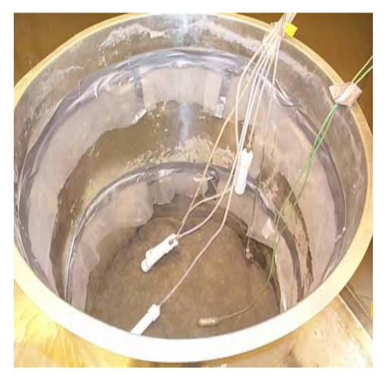
100 gallon stainless tank, PVC screened gas samplers, moisture sensors, two levels of baffle, gravel plenum, felt, copper line delivers methane
