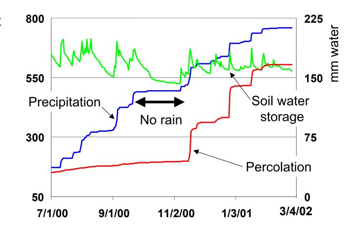
No evidence that defects in clay barrier healed when soil water increased
