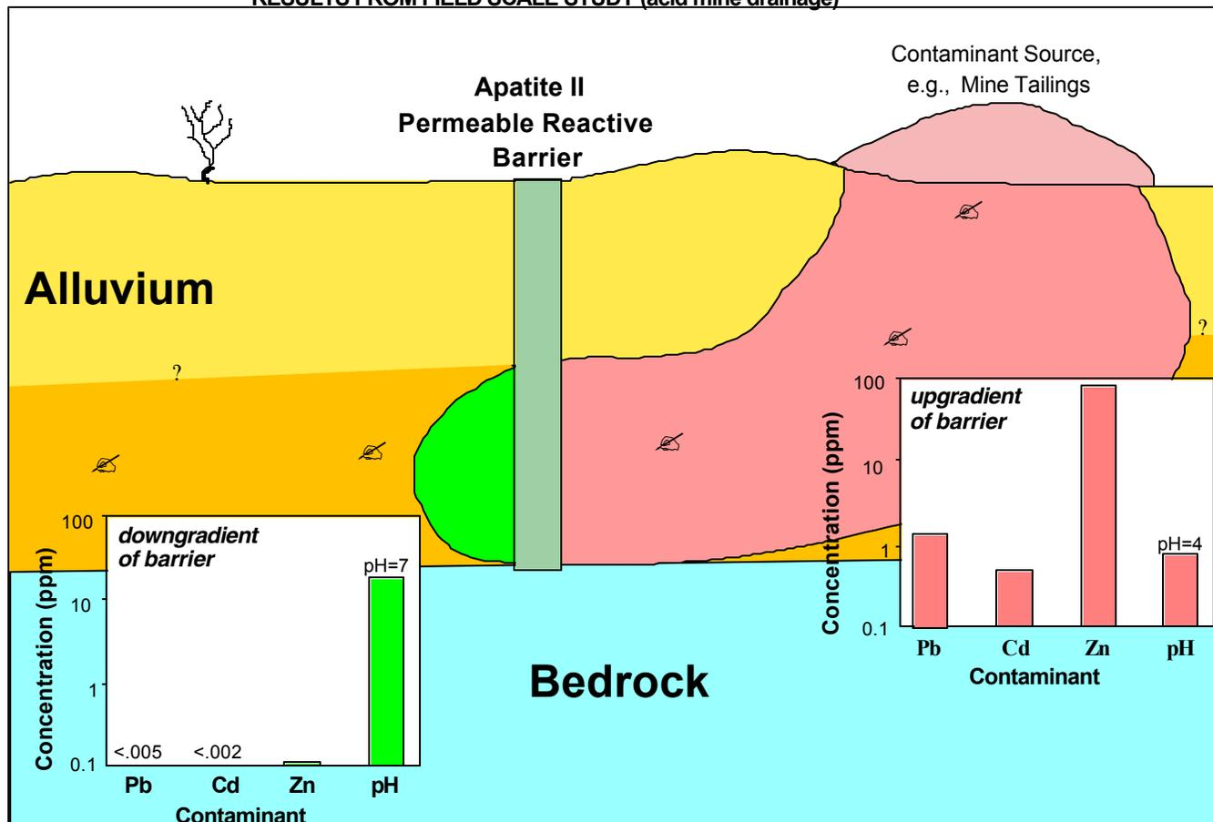
FIGURE 1. Schematic of a permeable reactive barrier showing actual results from the field.
