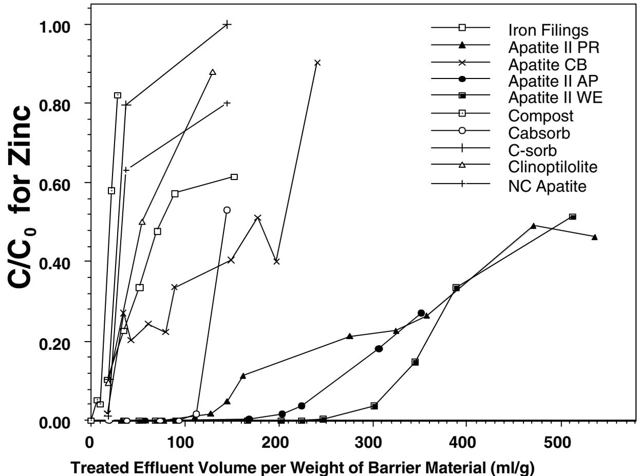
**FIGURE 2. Breakthrough of dissolved Zn through various permeable reactive barriers using contaminated groundwater from the Success Mine Site.  $C_{0zn} = 250$  ppm.**
