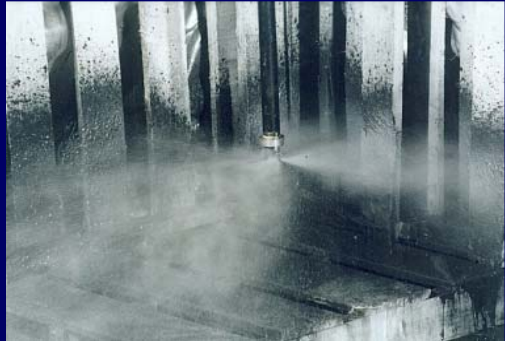
EZVI being atomized from injection nozzle
