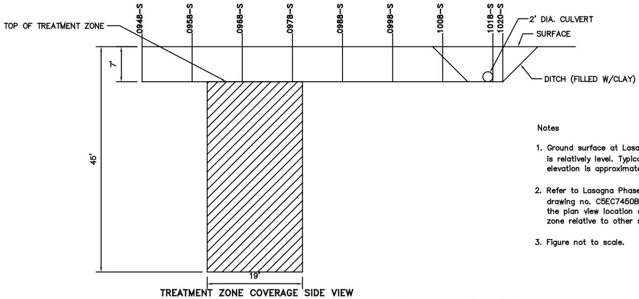
Figure 4.17 Final Configuration of Treatment Zone T-24
