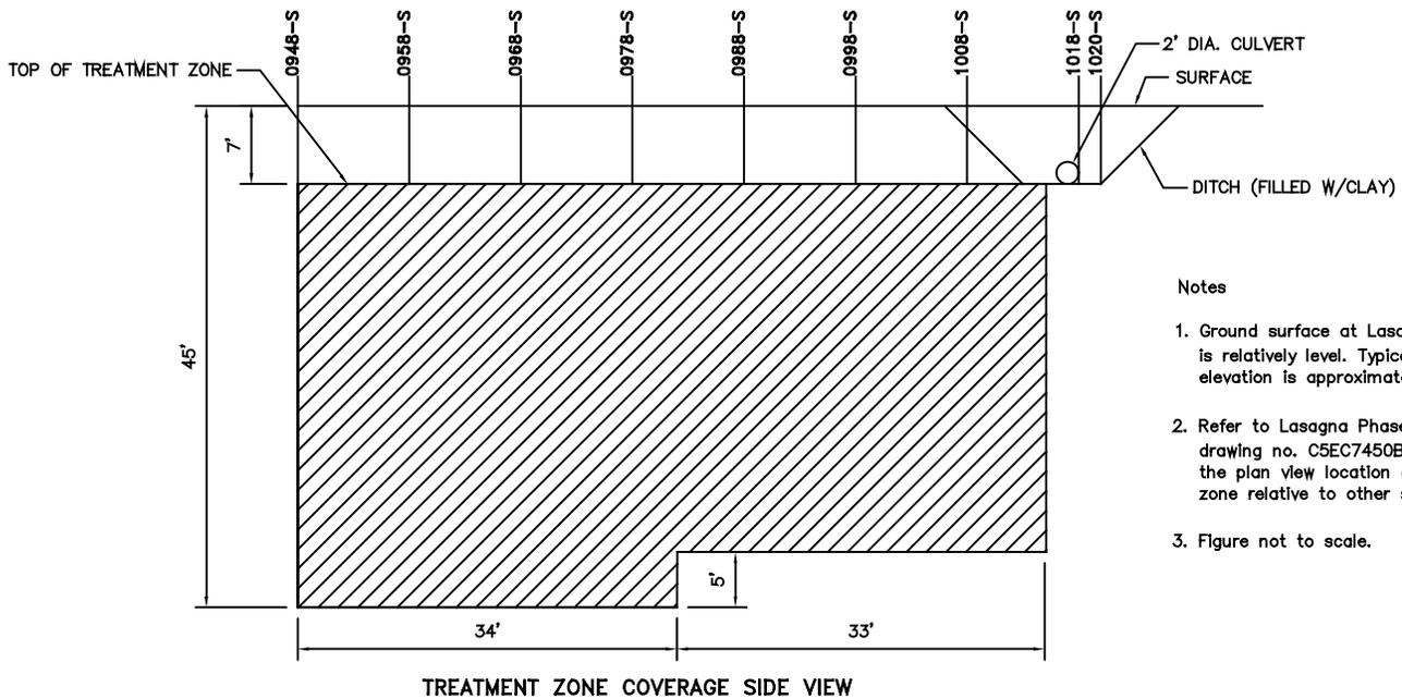
Figure 4.12 Final Configuration of Treatment Zone T-16
