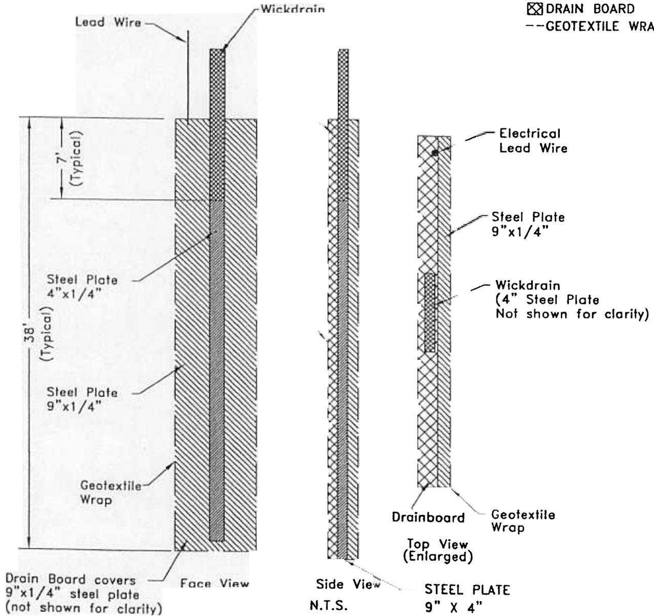
Figure 1.3 Typical Electrode Configuration
