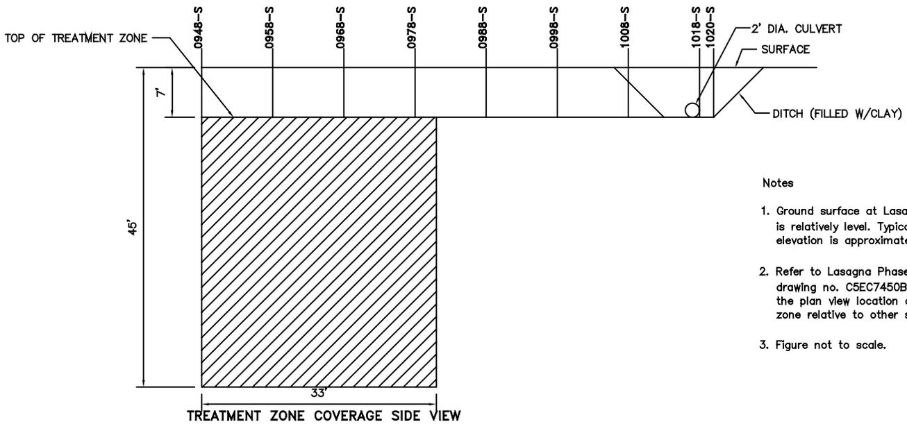
Figure 4.18 Final Configuration of Treatment Zones T-25, T-27, and T-28
