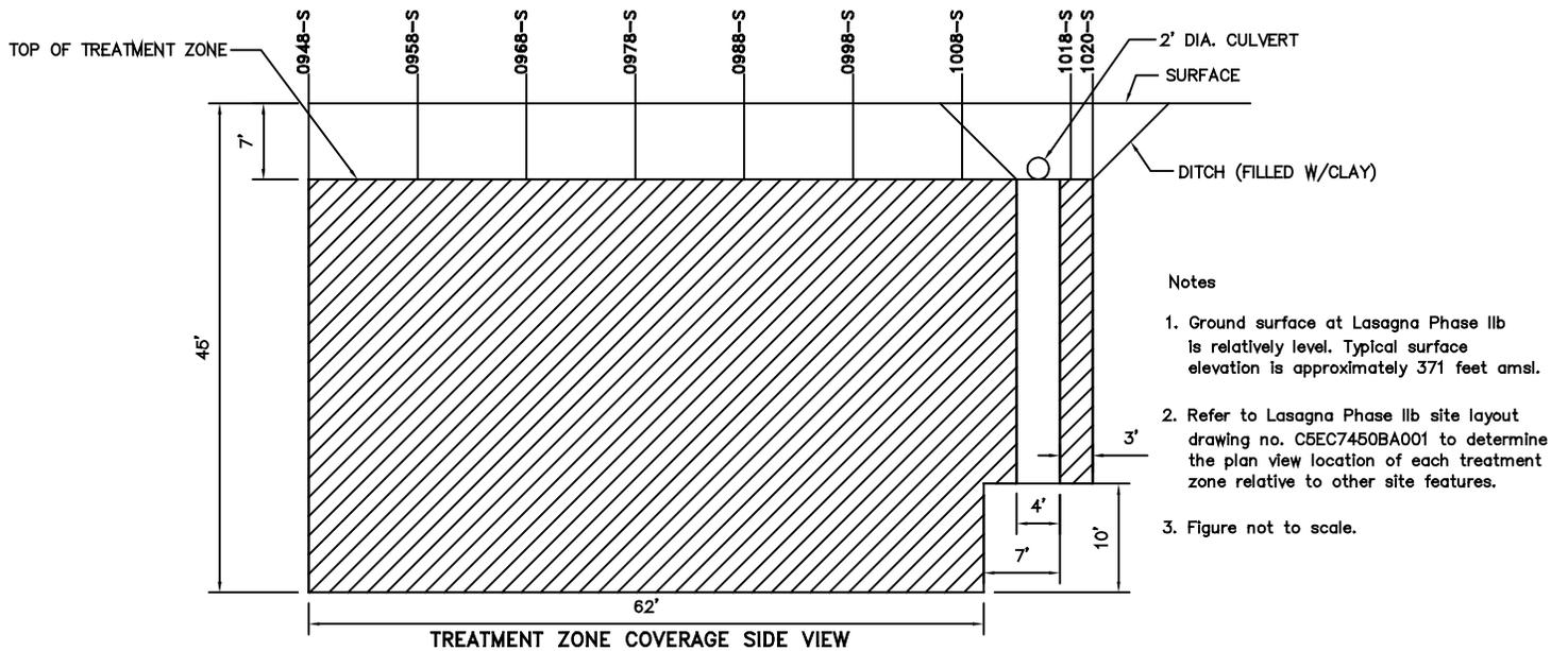
Figure 4.2 Final Configuration of Treatment Zones T-2 and T-3
