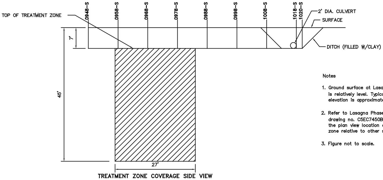
Figure 4.13 Final Configuration of Treatment Zone T-18
