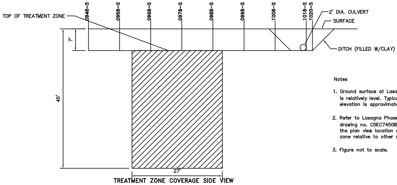
Figure 4.7 Final Configuration of Treatment Zone T-9
