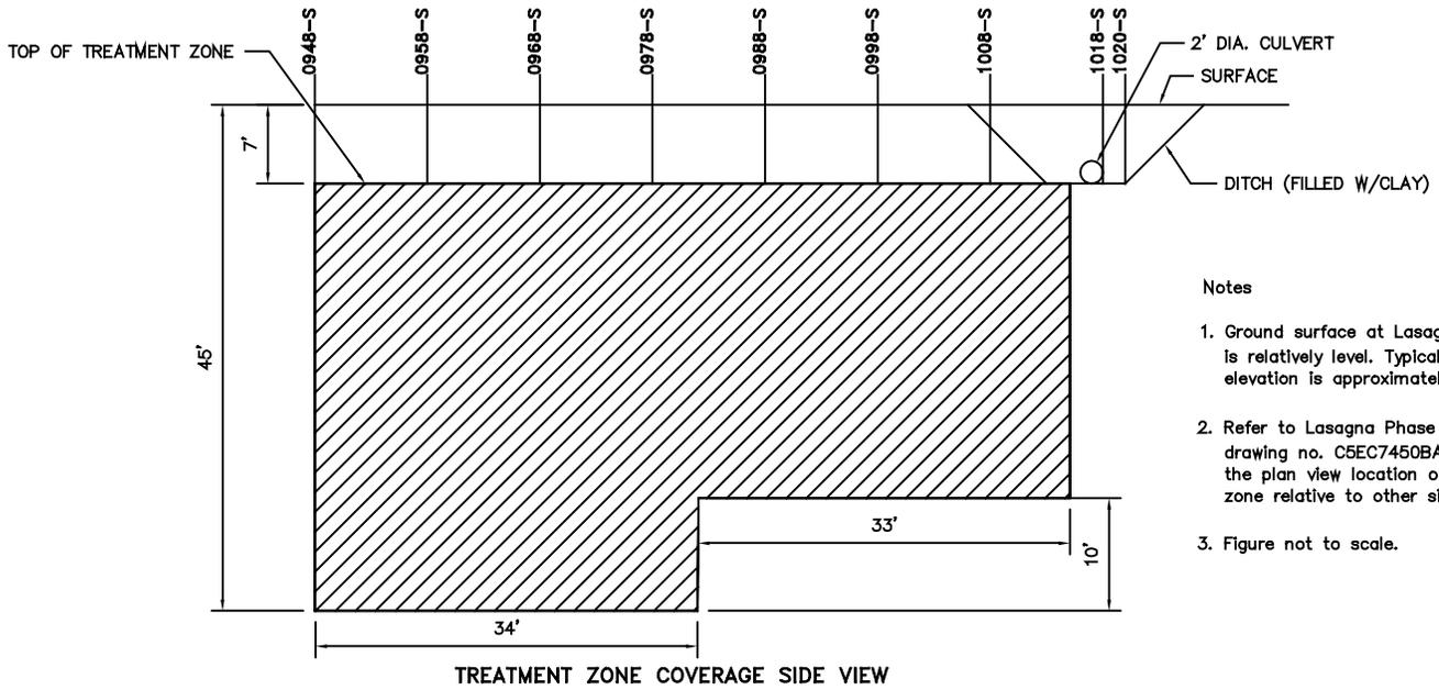
Figure 4.11 Final Configuration of Treatment Zones T-14 and T-17
