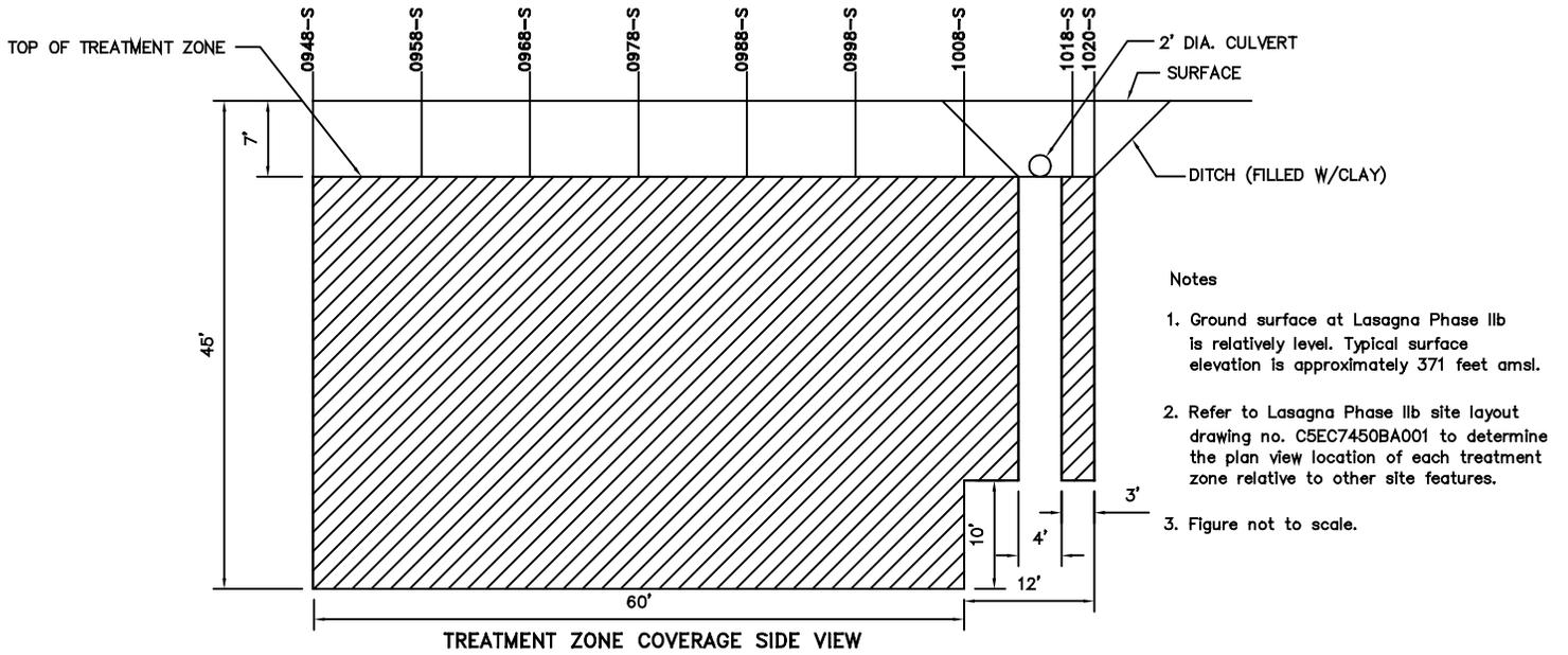
Figure 4.1 Final Configuration of Treatment Zone T-1
