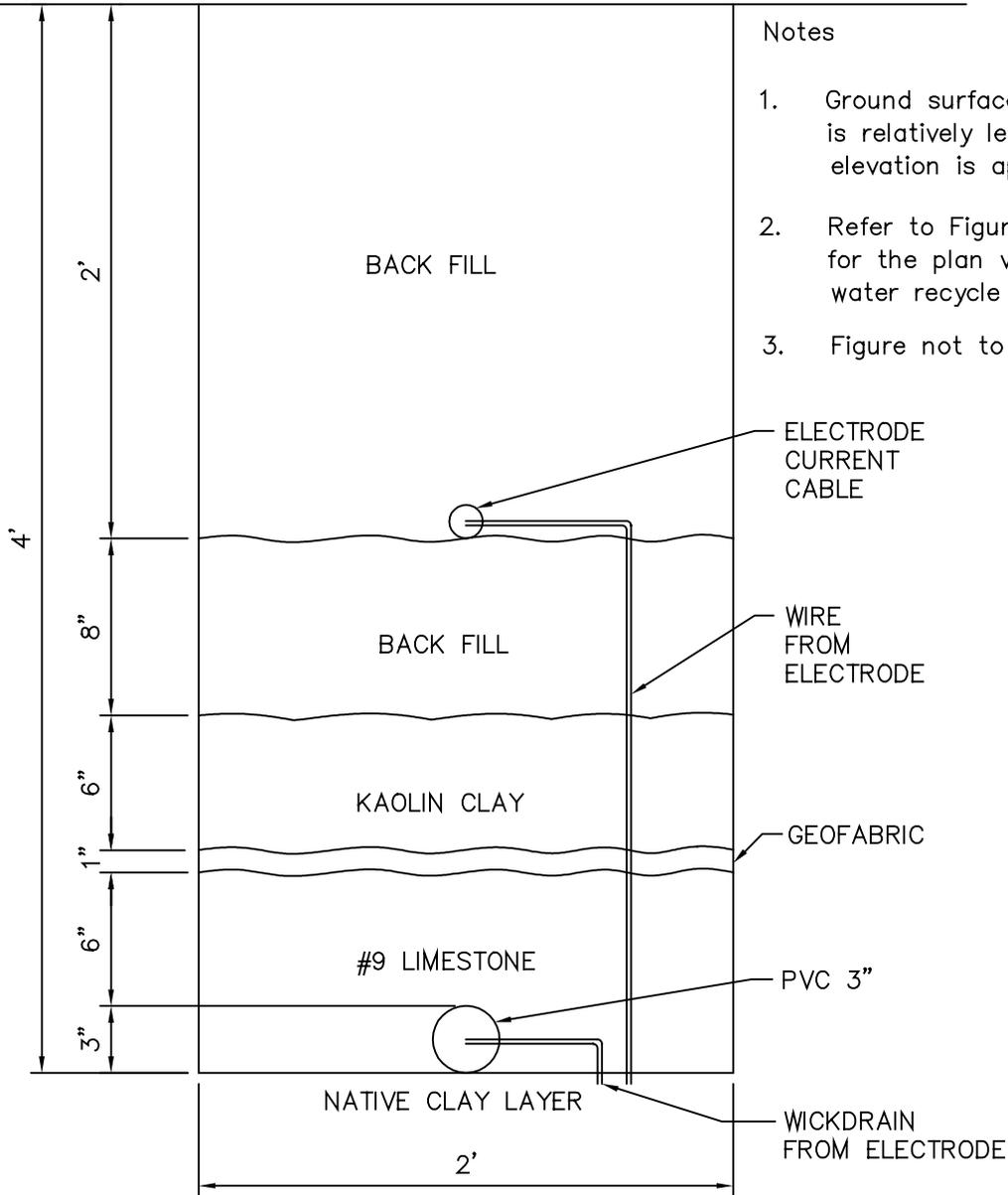
Figure 4.25 Typical Water Recycle System End View
