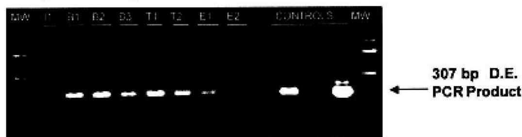
FIGURE 4. PCR Assay for the Detection Dehalococcoides -Like 16S rDNA in Groundwater Samples Taken from the Wells in the Pilot Test Area during Bioaugmentation Study.
