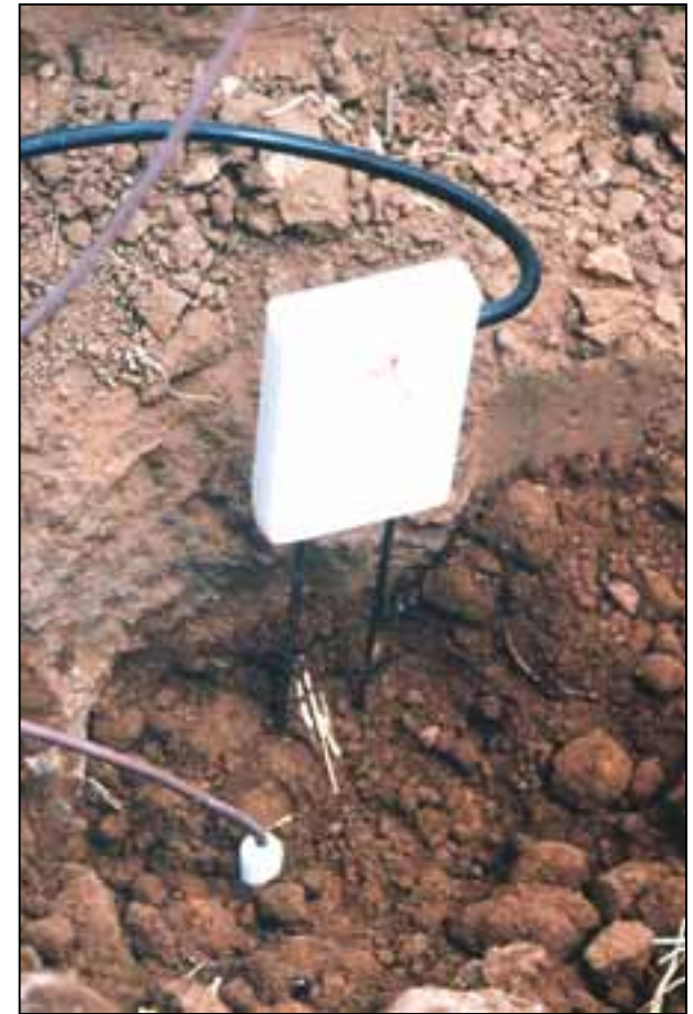
Water content reflectometer and heat dissipation unit
