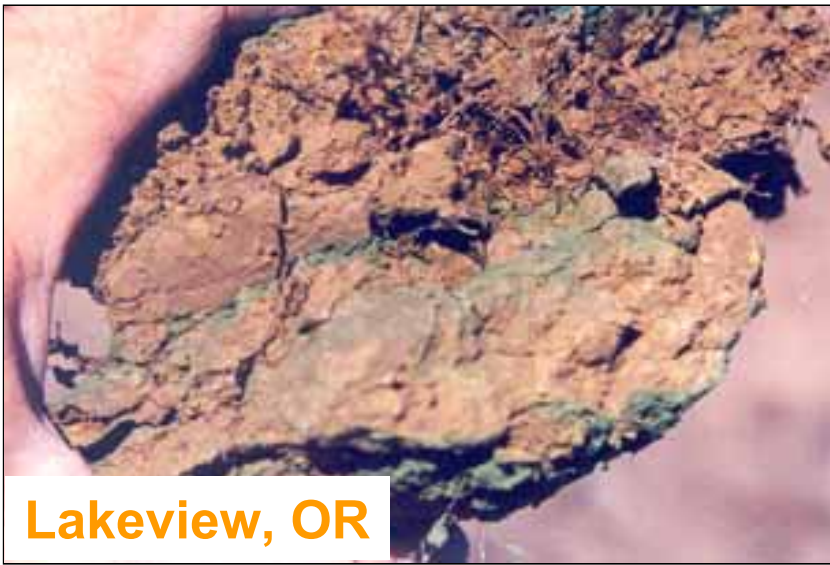
Test dye at structural planes
