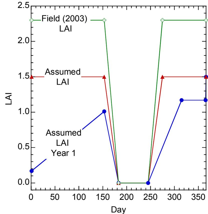
Properties of vegetation assumed during design relatively consistent with measurements
