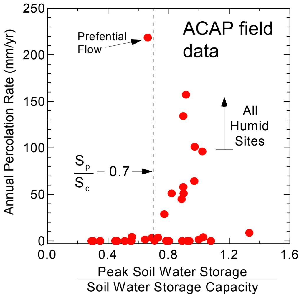
Storage capacity ( $S_c$ ) of ACAP covers computed assuming  $S_c = L\theta_{fc}$ , where  $L$  = cover thickness.
