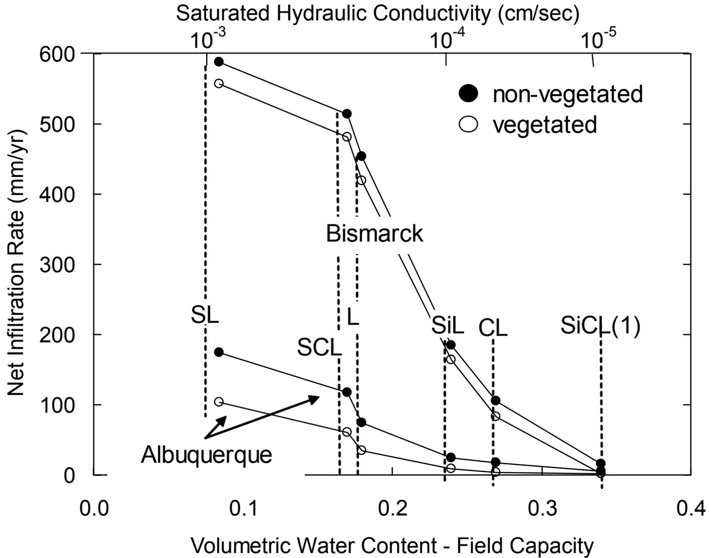
Finer textured covers transmit less percolation by enhancing runoff & retention
