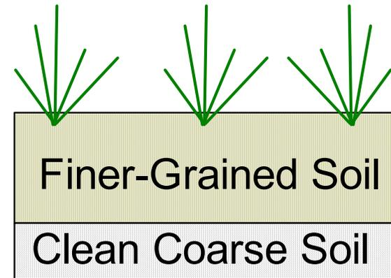
Capillary break can enhance storage capacity of the finer textured layer.
