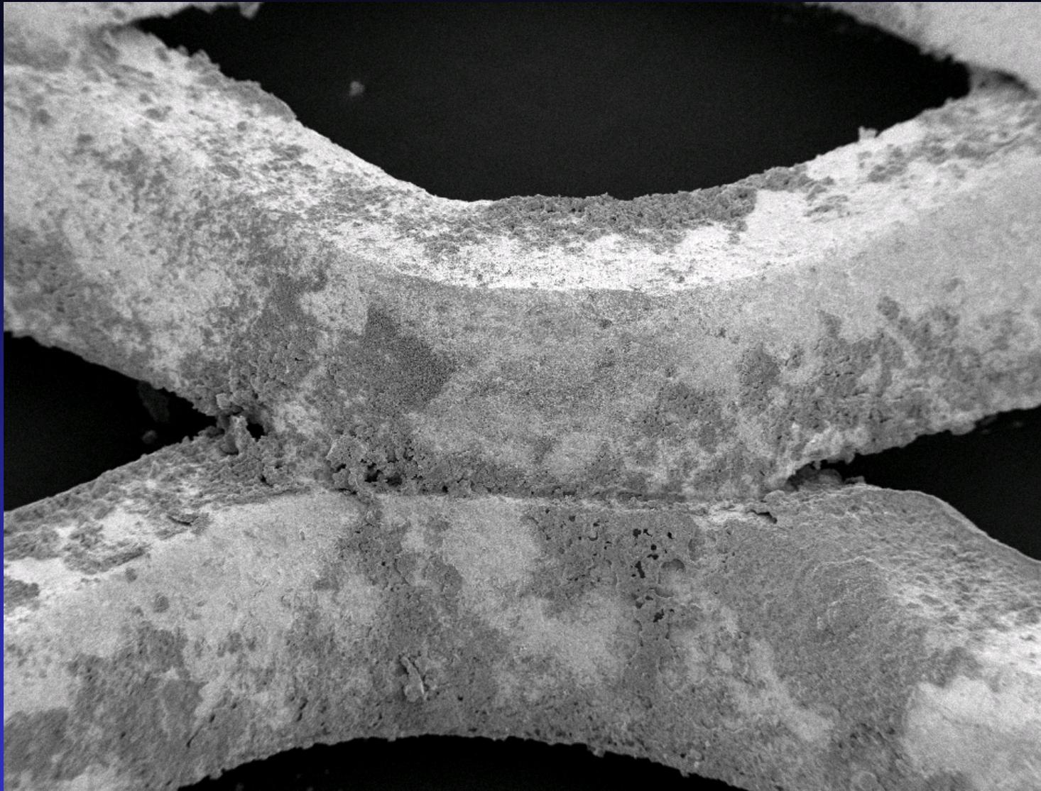
Scanning electron microscope image of a titanium mixed metal anode after 18 months of operation. Actual dimensions are 3 by 4 mm.
