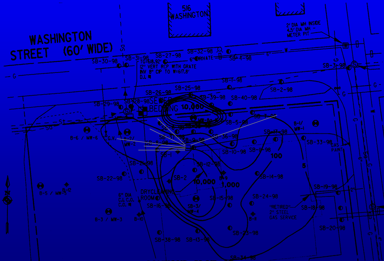
CONTOUR PLOT OF TETRACHLOROETHENE (PCE) IN GROUNDWATER (ug/L)
