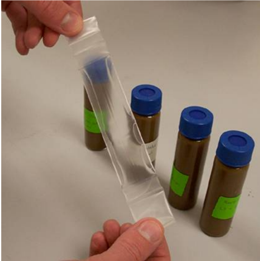
Semi-permeable membrane device
