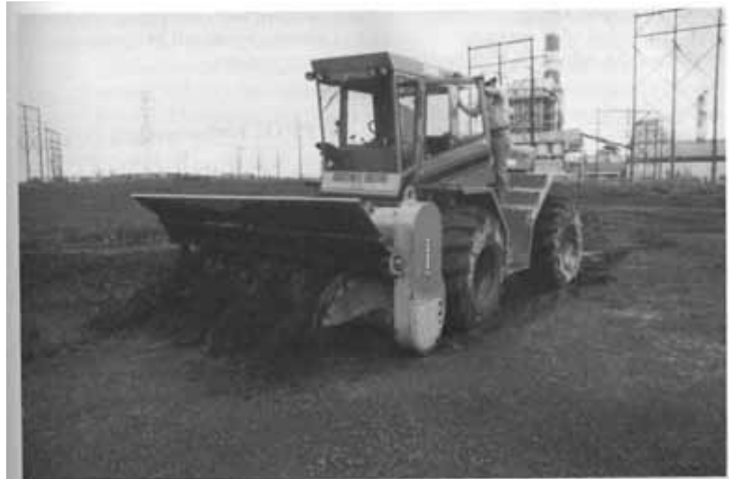
Figure 7-13 Auger-type sludge homogenization machine.
