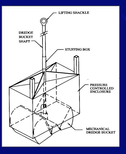
Pressure-controlled housing provides a dry environment around the mechanical bucket or mixing in-situ treatment zone
