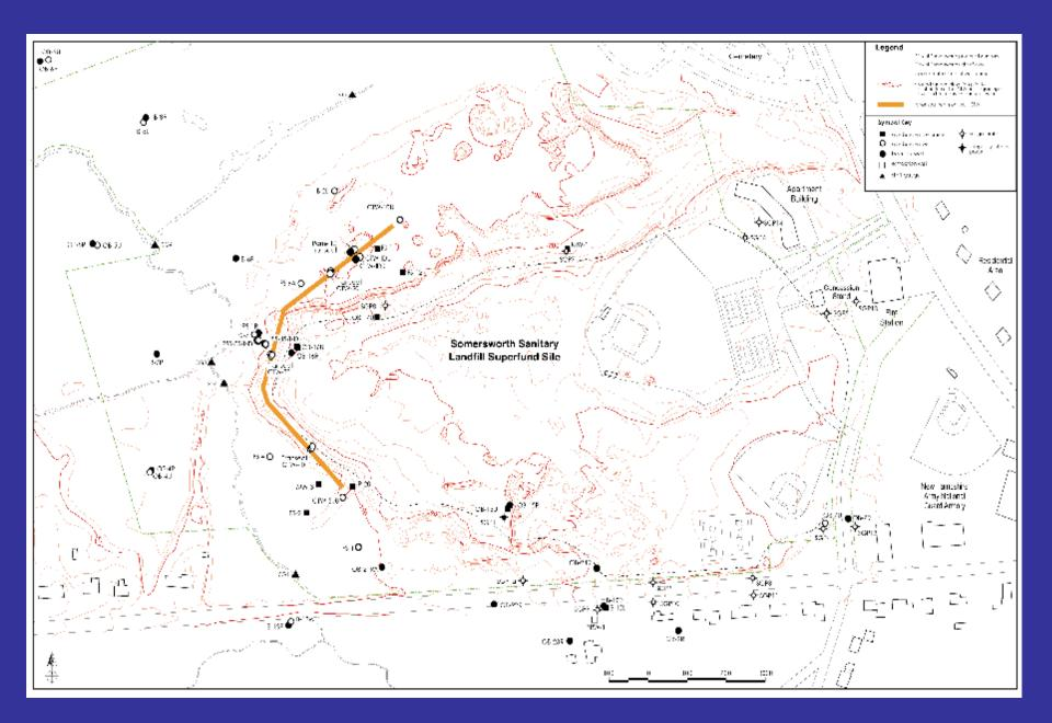
groundwater sampling at 30 monitoring wells for VOCs only 3times annually for several decades
