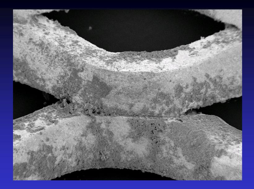
Scanning electron microscope image of a titanium mixed metal anode after 18 months of operation. Actual dimensions are 3 by 4 mm.
